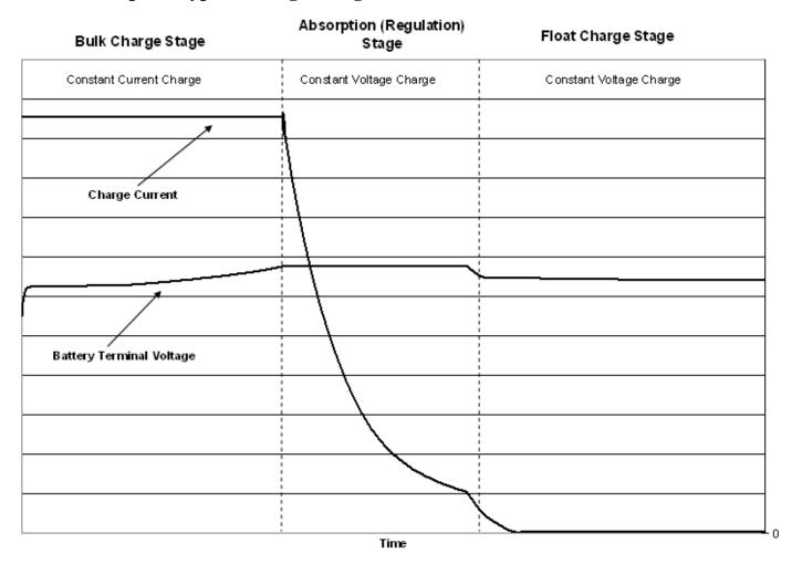
**Bulk Charge Stage** – Current is applied to the batteries at the maximum safe rate they will accept until voltage rises to near (80-90%) full charge level. The battery voltage rises because the charging current that is provided by the battery charger is replenishing its internal charge capacity. The charger current is flat (constant) and the battery voltage is rising.
